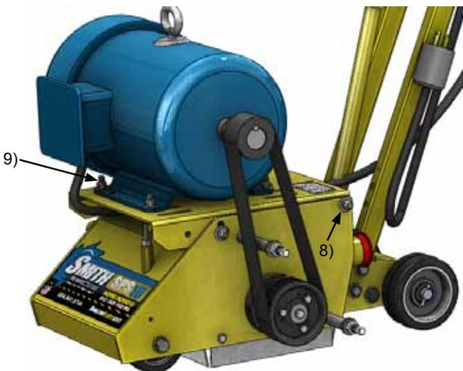
11. Roll the new belt on one groove at a time (two or single multi-groove belt) on both the top and bottom pulleys.
