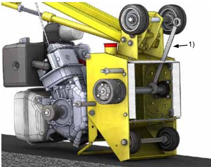
2. Remove the center screw using the 1/2" socket
